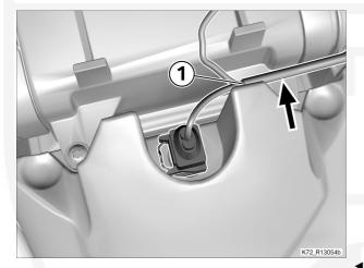
• Secure cable (1) for the air-temperature sensor (arrow).
